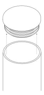
2. Slot the 76mm Post Extension into the top of the existing 76mm post and tighten the Grub screw to clamp the extension into place..
