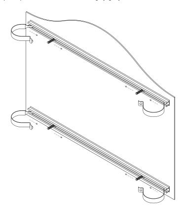
4. Place the Sign Panel with channel (Sign 1) against the posts and place the clips around the posts then connect it to the bolt. Then use the spacer and nut to tighten the sign in position.
