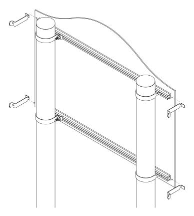
6. Slide the square head bolts into the channel railing of the back sign (sign 2)
